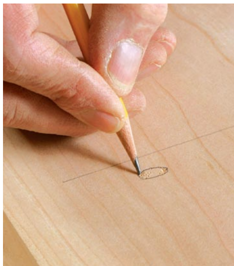
Outline the elongated holes and locate the position of the outside screws. With the points made by the scratch awl as a guide, use a pencil to scribe the elongated shape. If you anticipate the top is likely to expand, locate the pilot hole near the inside end of the elongated hole. If the top is expected to shrink, put the pilot hole near the outside end.
