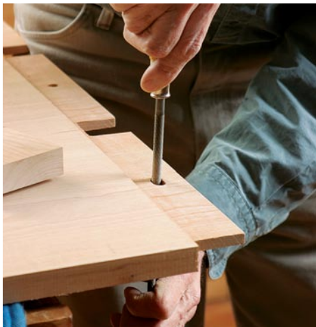
Elongate the holes. With the breadboard ends removed, use a marking gauge to scribe a pair of lines tangent to the end holes. A round file or rasp is ideal for elongating the end holes, but stay just inside the lines.
