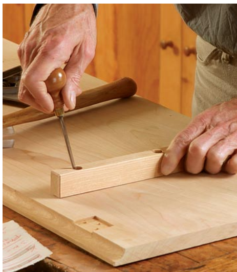
Mark the hole locations. Position the cleat on the underside of the top and mark the center of the middle hole. Make a series of points with a scratch awl to mark the elongated holes.
