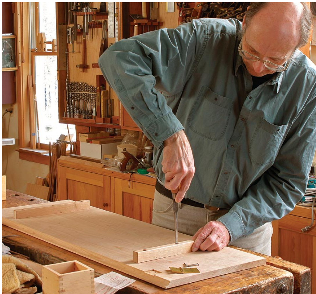
Drive the screws. After drilling pilot holes, drive the screws through the cleat until it's snug against the underside of the top. Don't use glue.
