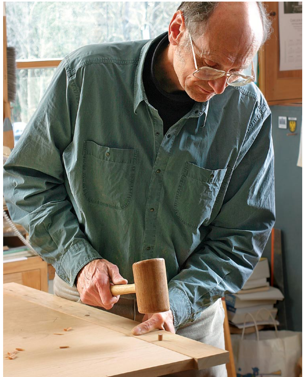
Drive the pins. Reassemble the breadboard ends after adding glue to the center tenon and mortise. Then add a thin coat of glue to each pin and drive them home. Trim the ends flush with the table.
