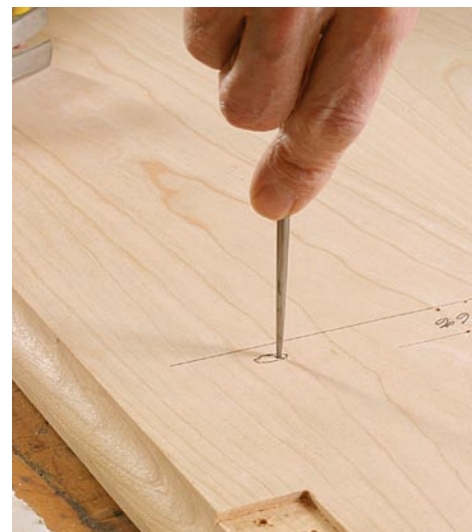
Outline the elongated holes and locate the position of the outside screws. With the points made by the scratch awl as a guide, use a pencil to scribe the elongated shape. If you anticipate the top is likely to expand, locate the pilot hole near the inside end of the elongated hole. If the top is expected to shrink, put the pilot hole near the outside end.
